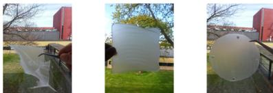
Films after solvent casting (Dimethyl formamide at 80 °C). PLA (left), PLA/CNF 5% (centre) and PLA/CNF/C30B 1% (right). The hybrid nanocomposites have great stability.
