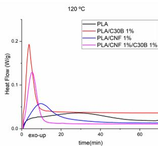
The PLA/CNF/C30B shows increased crystallization kinetic, furthermore it also shows a better spherulite distribution (not showed here). Both CNF and C30B appeared to have a similar effect of RAF development.
