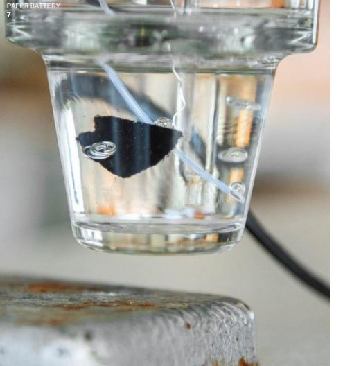
A paper battery is a power source using nanotechnology to store electricity in a cellulose fibre material.
