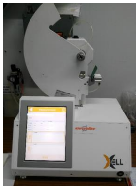
Figure 6 - Elmendorf pendulum 4000mN used to determine tear resistance.
