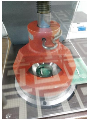
Figure 5 - Adamel Lhomargy EC 0.5 used for burst index determination.
