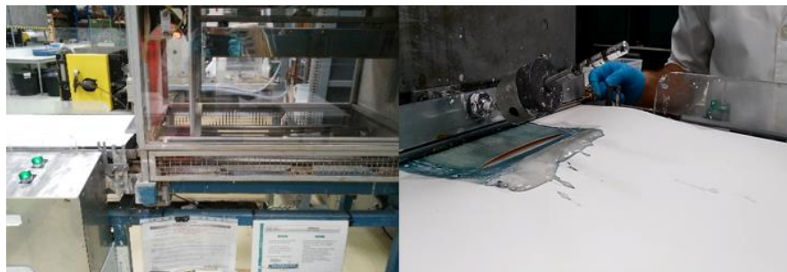
Figure 1 - Blade coater equipped with an infrared section (Endupap).
