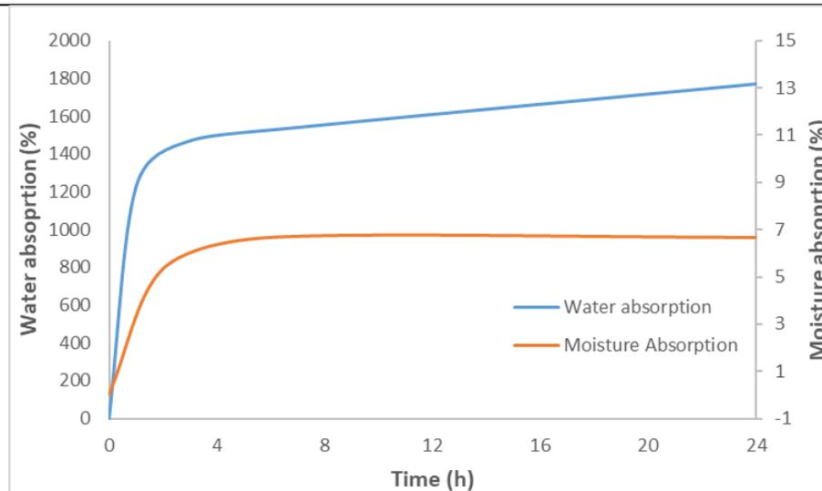
Fig. 6. Water and moisture absorption values for CNF aerogels
