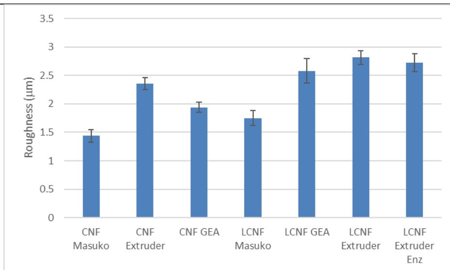
Fig. 2. Surface roughness measured with laser profilometry
