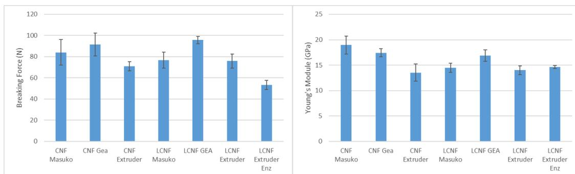
Fig. 1. Mechanical properties of CNF and LCNF films.
