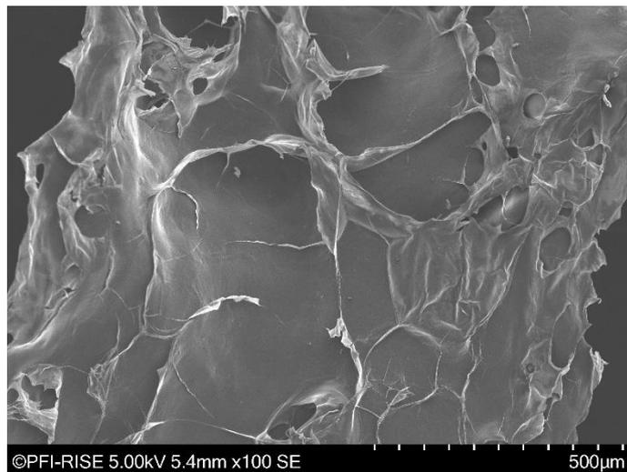
Fig. 5. SEM image of a freeze-dried CNF.
