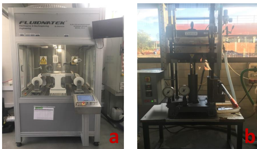
Figure 2. Electrospinning equipment (a) and hydraulic press (b)
