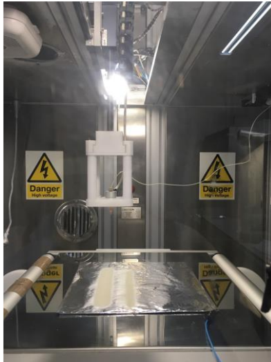
Figure 5. Preparation of the fibrous mats
