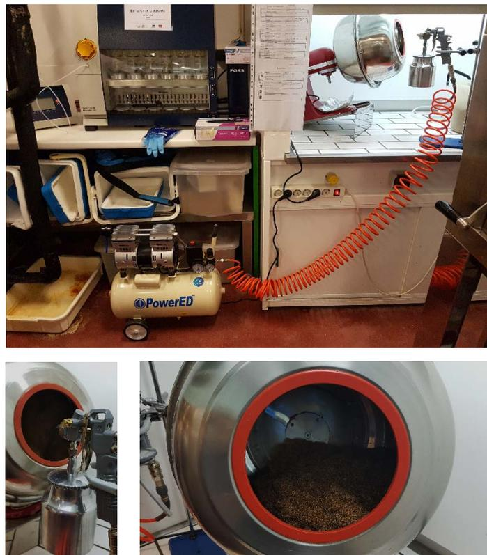
**Figure 2** Overview of the setup used for the fibers functionalization (upper image) with detail of the air spray gun (bottom left image) and of the rotating drum (bottom right).
