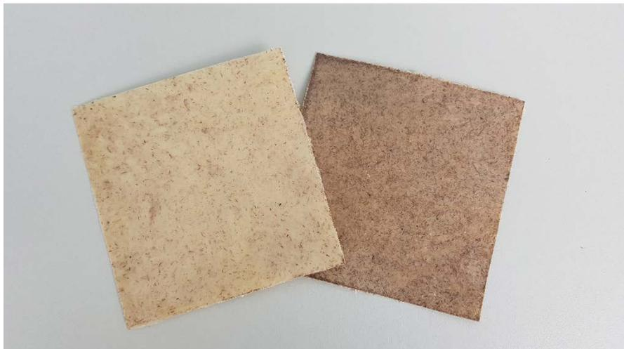
**Figure 6** Green composite sheets with low (left) and high (right) natural fiber contents.
