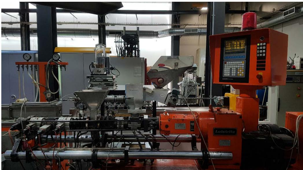
**Figure 3** Twin-screw extruder used to prepare the green composite pellets.
