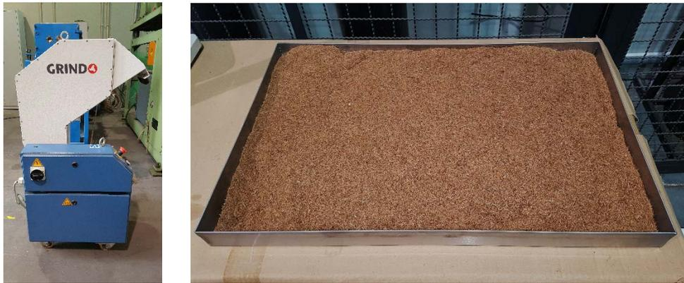
**Figure 1** Granulator (left image) used to chop the fibers and the resultant fibers after sieving prior to drying in a tray (right image).
