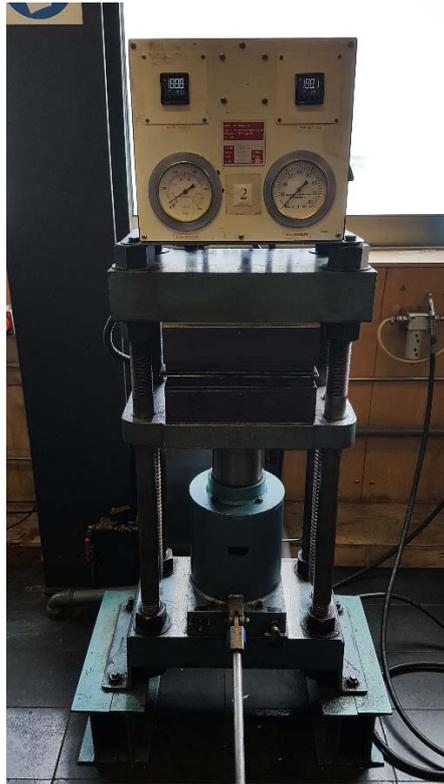
**Figure 4** Hydraulic press used to prepare the green composite sheets.
