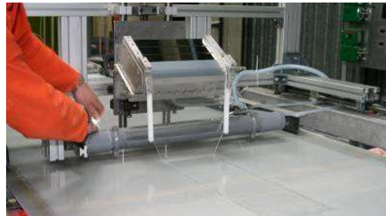
CTP's curtain coater located above Grenoble INP Pagora's paper machine
