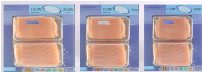
Photographs of oxygen indicator ink printed on a MAPed food package.
