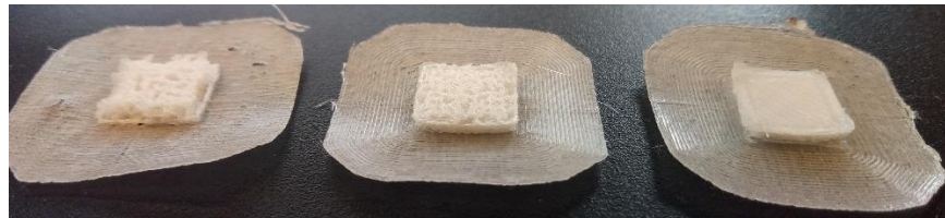
Figure 4. BioPE with 10% TMP cube samples during 3D printing conditions optimization.
