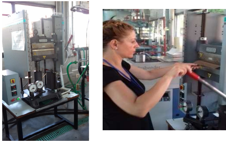
Figure 2. Preparation of the films of PLA and PLA+AU from the electrospun mats on hydraulic press 4122-model
