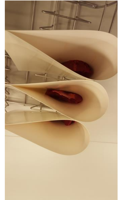
Figure 1: Meat packaging trial in oxygen scavenging material, Stora Enso
