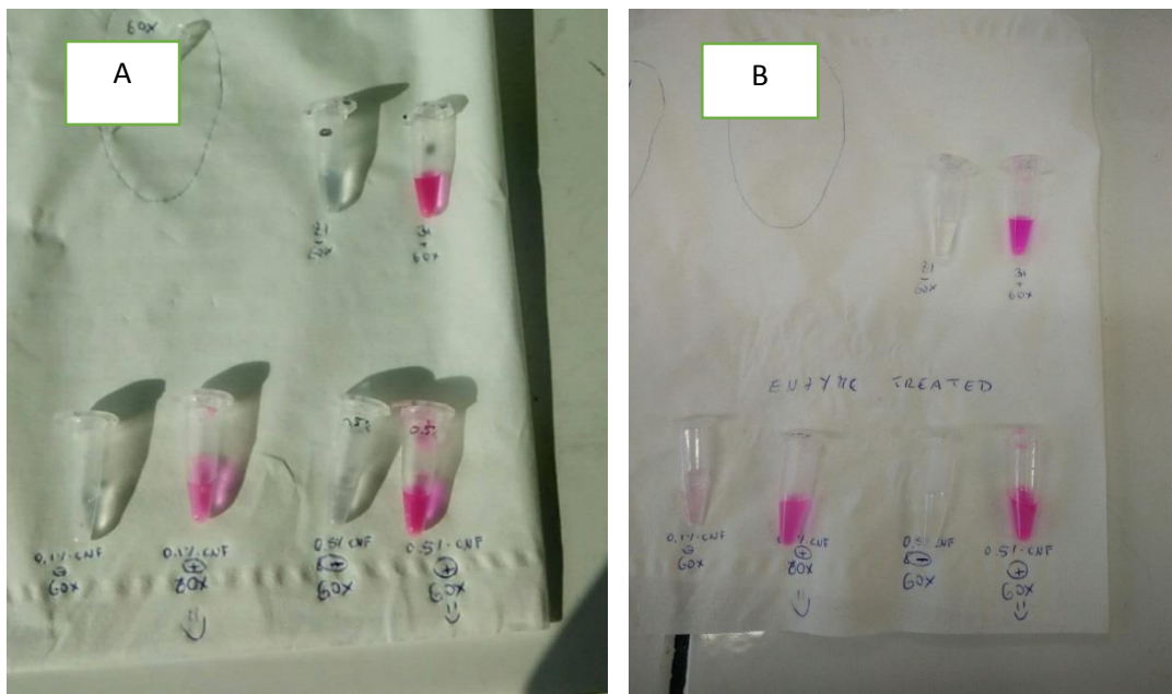
Figure 1: Amplex Red assay: (A): top row: blank without CNF-T - without GOx, with GOx, bottom row: CNF-T (0.1%) without GOx, with GOx; CNF-T (0.5%) without GOx, with GOx; (B): top row: blank without CNF-E – without GOx; with GOx; bottom row: CNF-E (0.1%) without GOx, with GOx; CNF-T (0.5%) without GOx, with GOx
