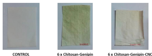
Figure 12: Macroscopic effect of 6 chitosan-genipin and chitosan-genipin-CNC coatings on non-calendared paper.
