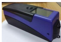
Figure 11: SpectroEye portable spectrophotometer
