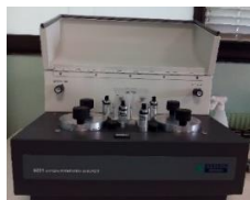
Figure 10: M8001 oxygen permeation analyser acquired on Systech ILLINOIS.
