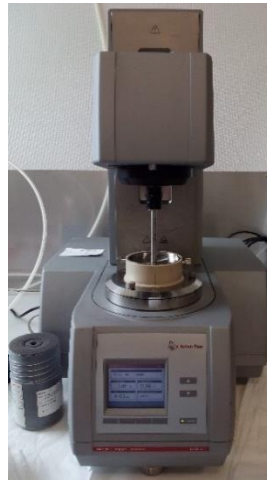
Figure 5: Modular compact MCR 302 rheometer supplied by Anton Paar.
