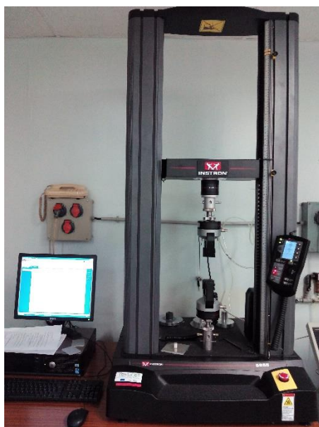
Figure 18: Instron 5965 apparatus used to measure the mechanical influence of each tested coating on paper samples.
