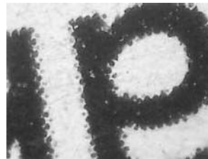
Typical print result: tiny „sawtooth“ at edges
