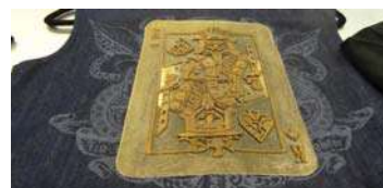
S.P. on T-Shirt several subsequent print runs with intermediate drying Source: own photograph at SGIA print workshop
