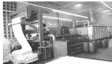
Rotational S.P. on textile web with steam dryer
