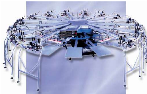
M&R "Terminator" up to 16 printing units, 6m diameter
