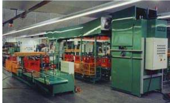
FK 08-27 / 47 Fully automated multicolor press for beer cases 800 per h
