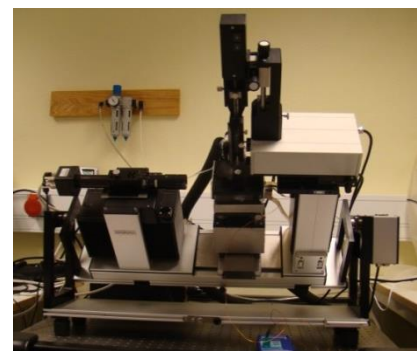
Figure 3. Contact angle measurement machine. Tilted at 45°.
