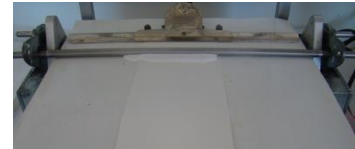
Figure 1. Coating of a suspension with the rod coater
