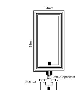
Antenna design depends on the frequency, but will be tuneable to a small degree by having an adjustable capacitance.
