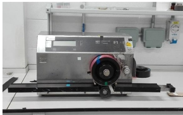
Figure 3: IGT Flexographic Printability Tester F1.
