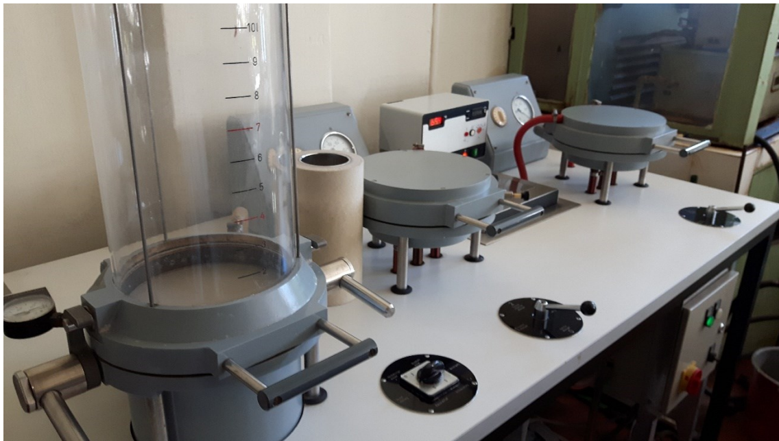
Figure 1: Laboratory paper machine
