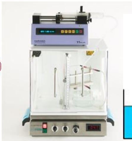
Var V1 (Nisco, CH) - electrostatic capsule generator
