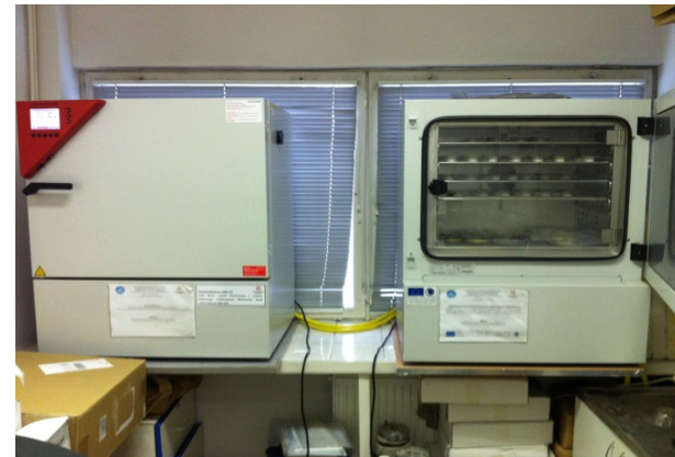
BINDER KBF115 (Niemcy) Climatic chamber - different sizes
