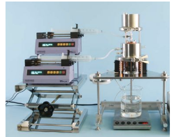
Var D Generation II (Nisco, CH) - electromagnetically driven generator
